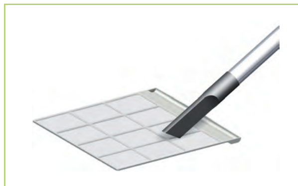
Fig. 16: Cleaning with a vacuum cleaner
